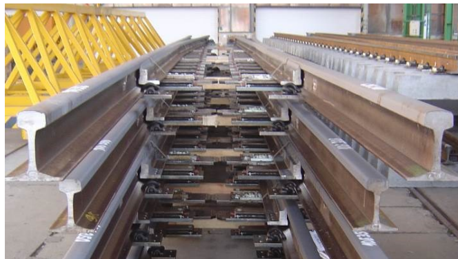
Figure 22 - Complete half-switch panels stacked
