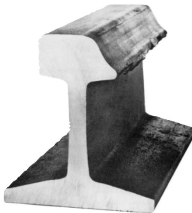
Figure 38 – Lateral wear of the rail head
